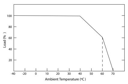
• If being used in higher ambient temperatures, ensure the load on the LED driver is de-rated in accordance with this chart. Failure to do so could lead to a premature failure, which is not covered by the warranty.
